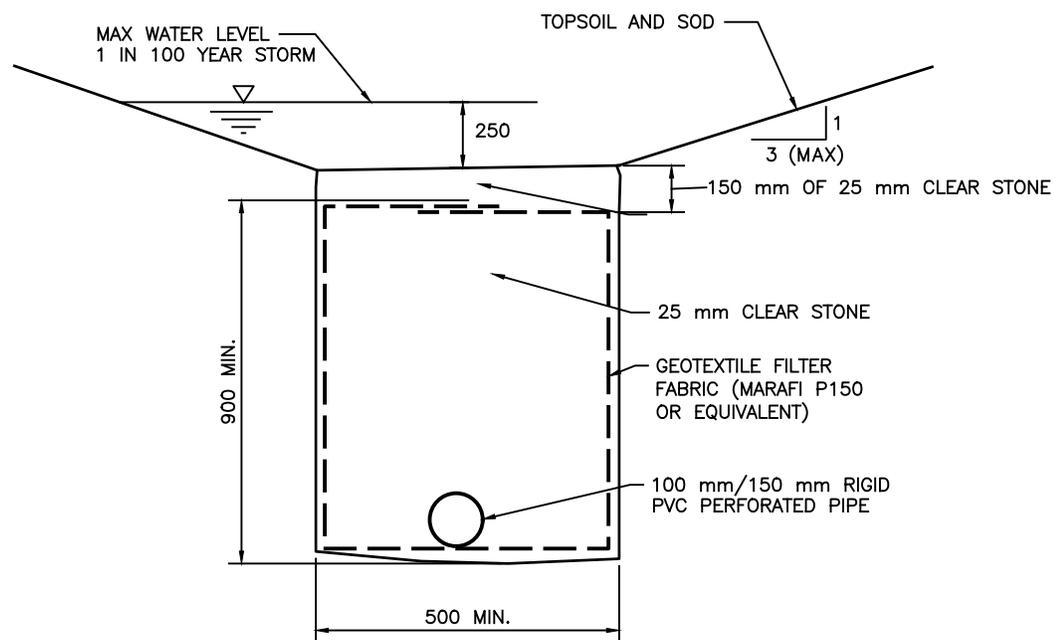
SWALE AND UNDERDRAIN CROSS SECTION
