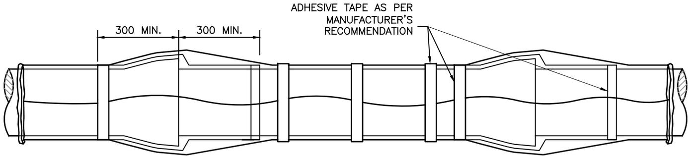
ONE LENGTH OF V-BIO ENHANCED POLYETHYLENE (OR APPROVED EQUIVALENT) FOR EACH LENGTH OF PIPE, OVERLAPPED 300 mm AT JOINT.
