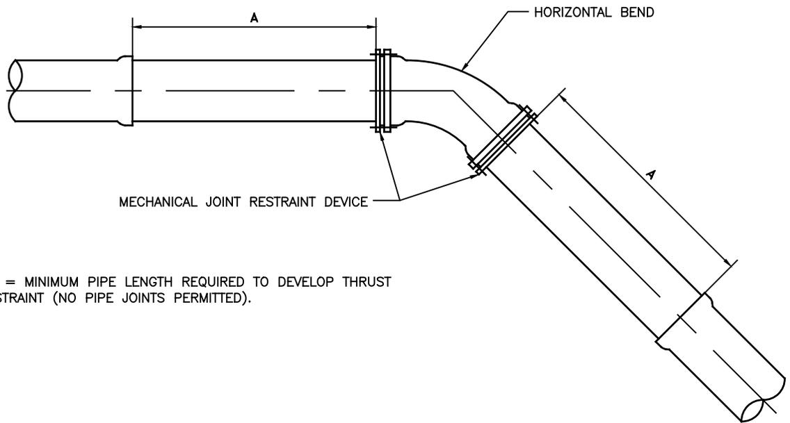
"A" = MINIMUM PIPE LENGTH REQUIRED TO DEVELOP THRUST RESTRAINT (NO PIPE JOINTS PERMITTED).
