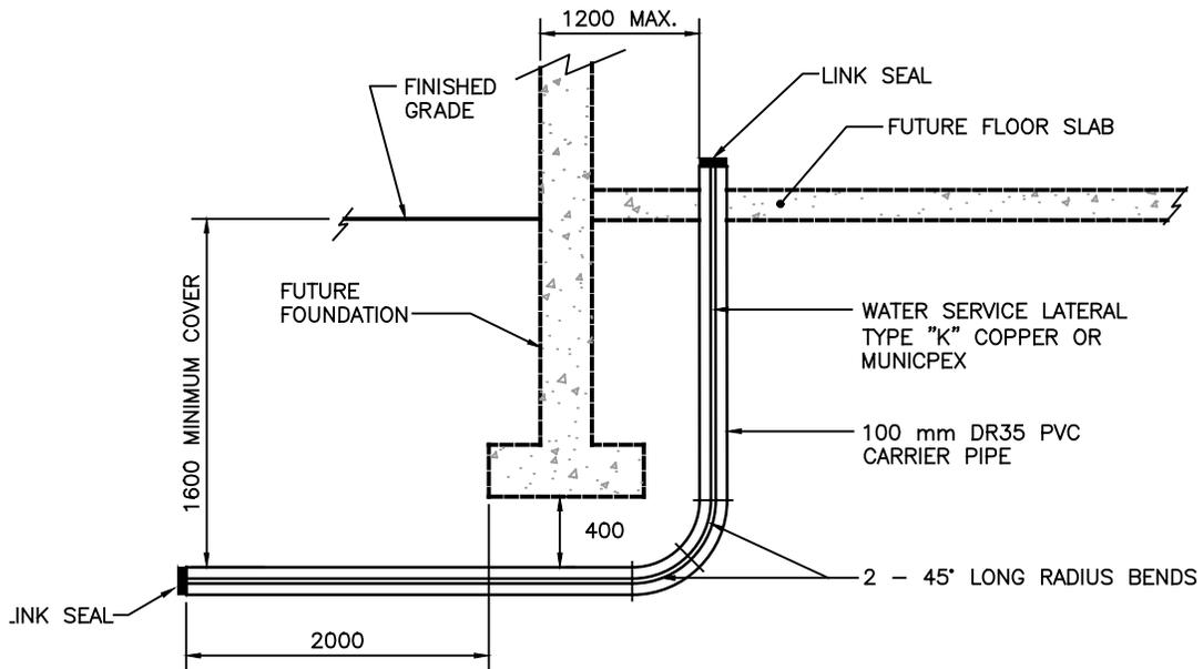
CARRIER PIPE INSTALLED PRIOR TO FOUNDATION INSTALLATION
