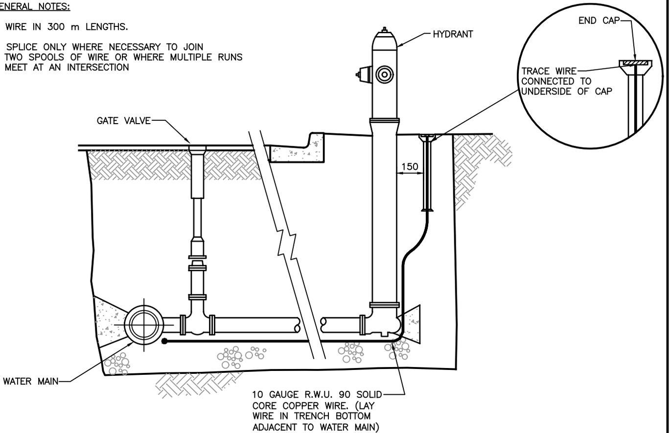
10 GAUGE R.W.U. 90 SOLID CORE COPPER WIRE. (LAY WIRE IN TRENCH BOTTOM ADJACENT TO WATER MAIN)
