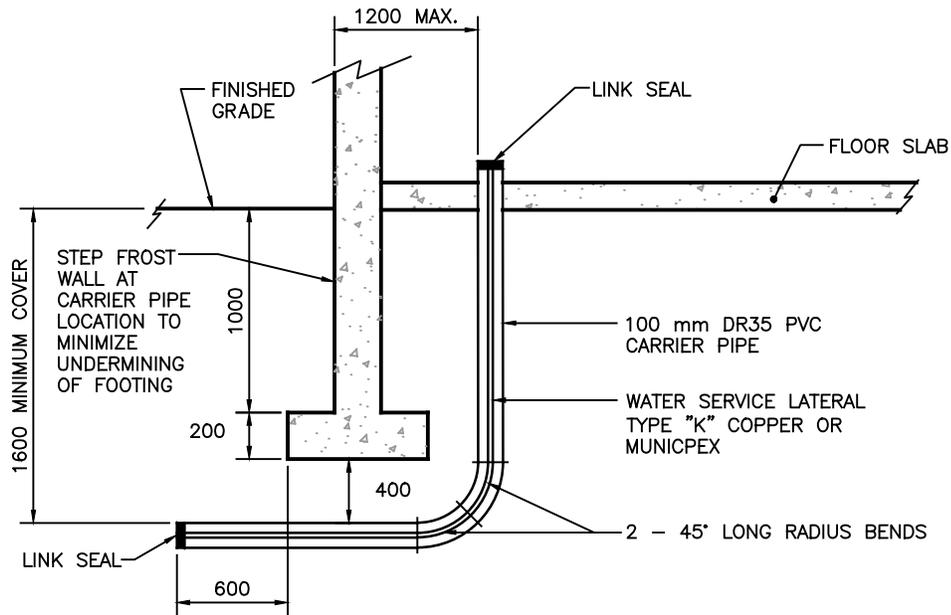
CARRIER PIPE INSTALLED AFTER FOUNDATION INSTALLATION
