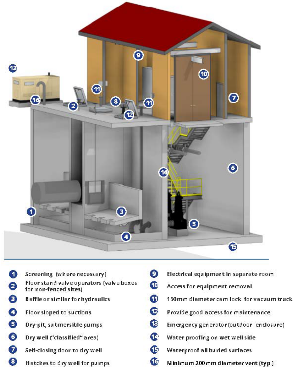
Figure 4.4: General Arrangement - Large Pumping Station
