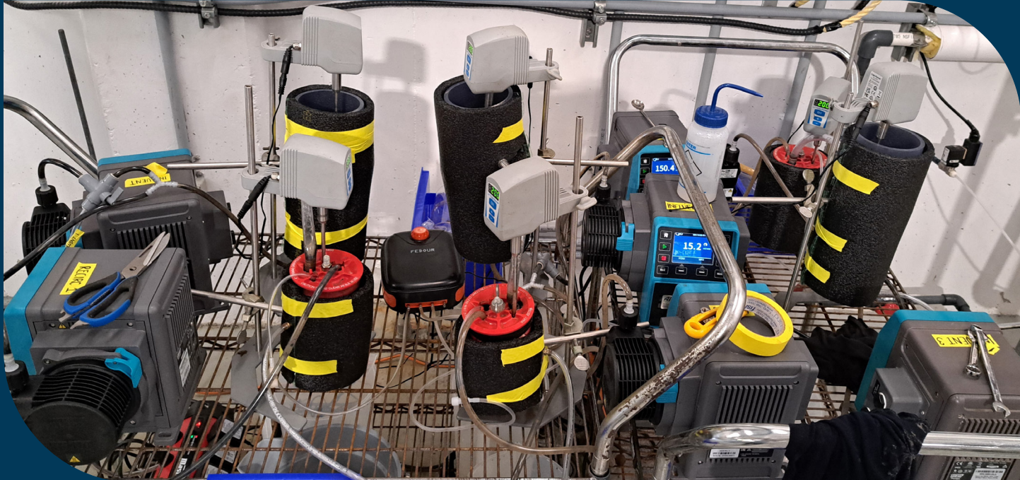
Biological Aerated Filtration (BAF) Pilot Testing
