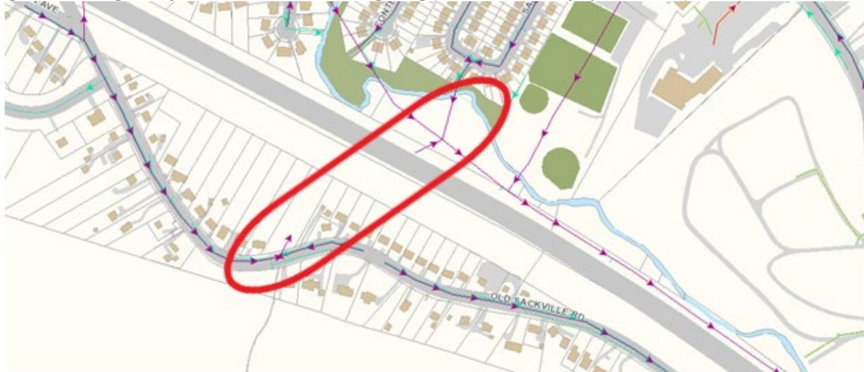
Normally this sort of missing culvert information would result in the model failing to run due to a ‘missing outfall error’ during initialization, triggering an investigation immediately. This case was somewhat unique as the local flat topology of the floodplain allows the flows within the pipes on Old Sackville Road to reverse (flow against grade) to the northwest and back to the system at Crystal Court. During dry weather simulations, this does not even cause a surcharge.
