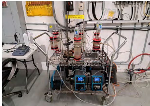
Small-Scale Biological Aerated Filter Study
