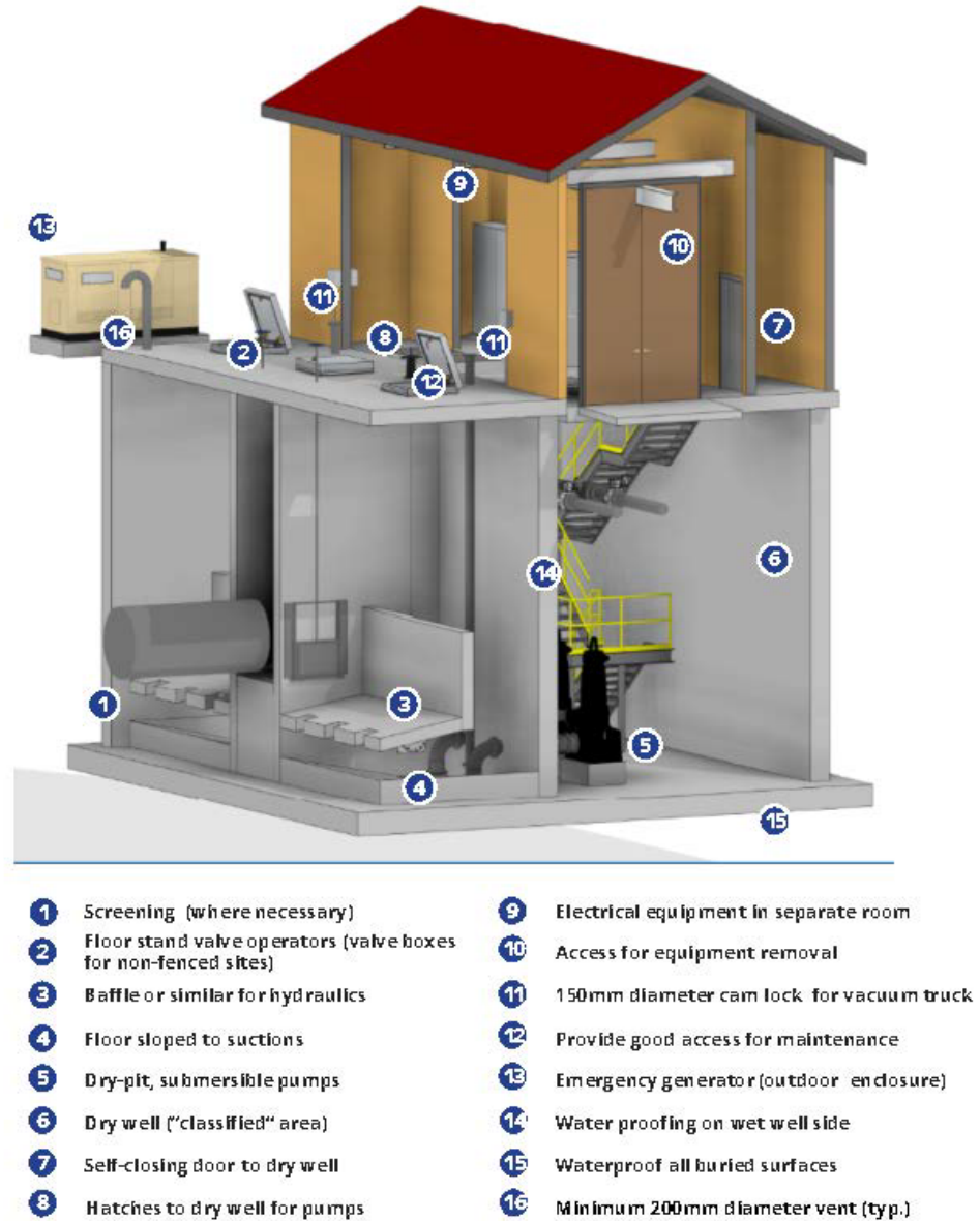
Figure 4.4: General Arrangement - Large Pumping Station
