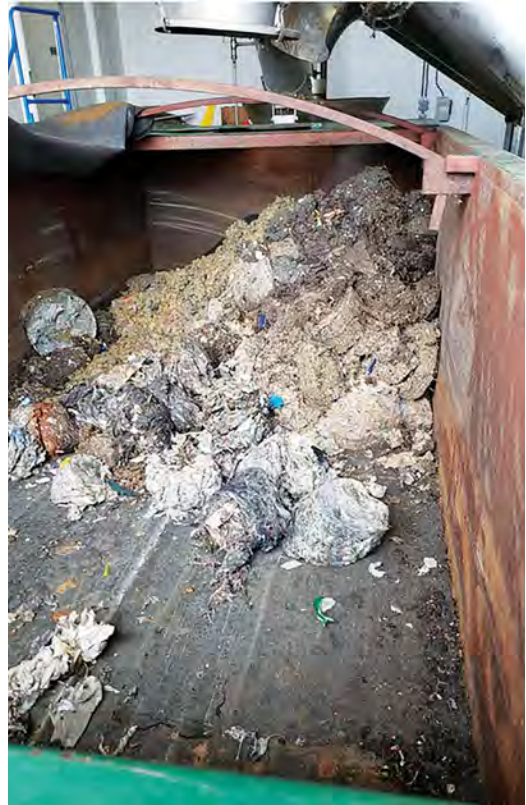
Figure 5: Compacted and dewatered screenings from DWWTF.
