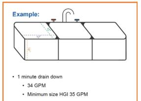
The peak flow rate for a 3-compartment sink, measuring 17" x 17" x 12", and using 75% of the volume of each compartment, would be as follows:
