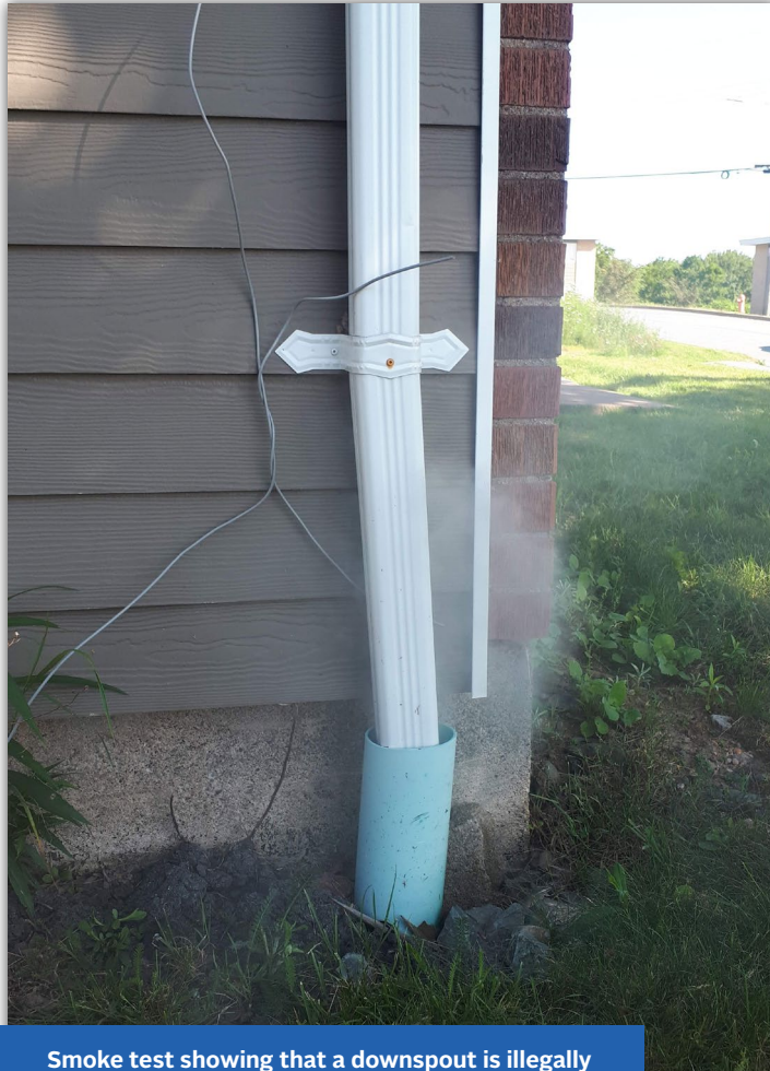
Smoke test showing that a downspout is illegally connected to the Halifax Water wastewater system
