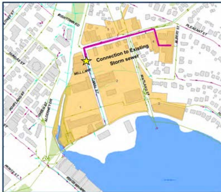
Figure 2-4: Sewer Separation Scenario for Canal Street
